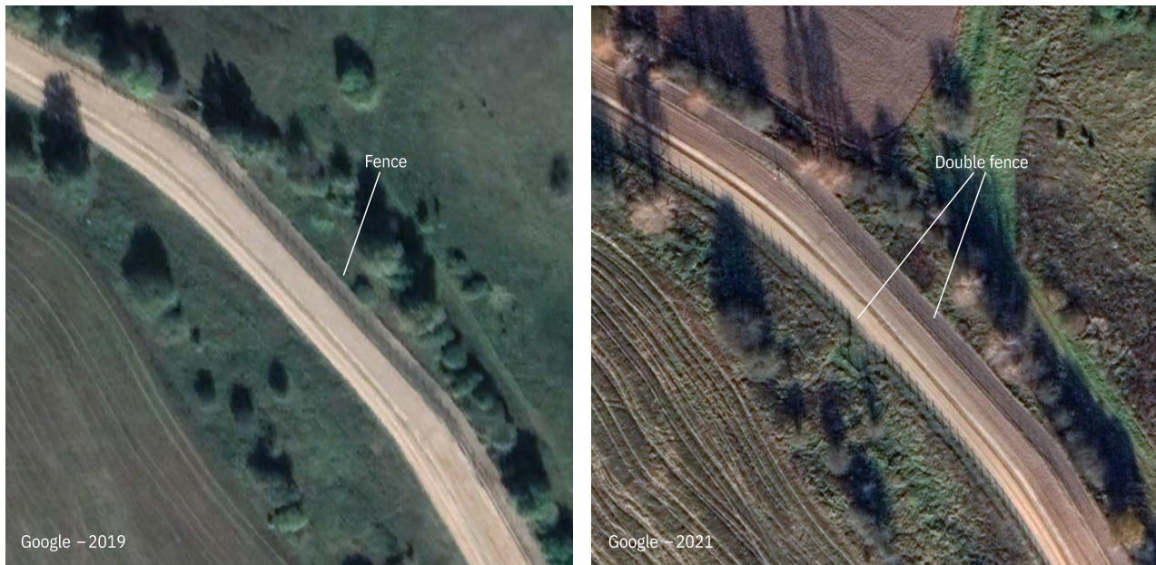
Figure 17. Satellite imagery analysis detected a doubling of the Sistema fencing layer along sections of the Belarusian side of the border in recent years. Satellite Imagery: Google Earth Image ©2019/2021 Maxar Technologies, and Google Earth Image.
